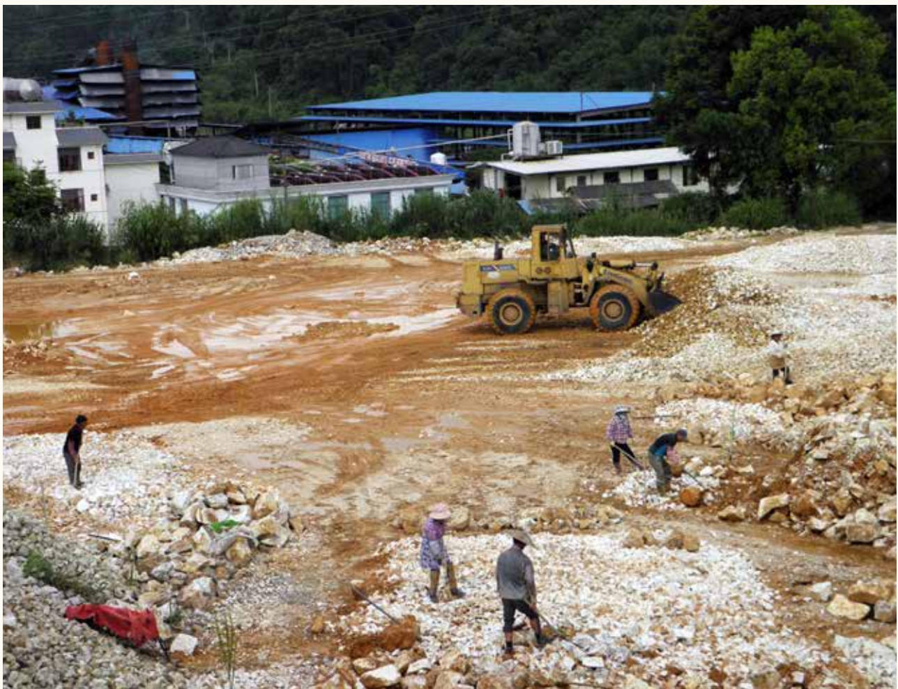
Workers are smashing quartzite stones at the field of a silicon plant in Nujiang, Yunnan province, China. The buildings behind are the workshop, where the big stacks are connected to furnaces for silicon purification. (Photo by Zanxin Wang)
